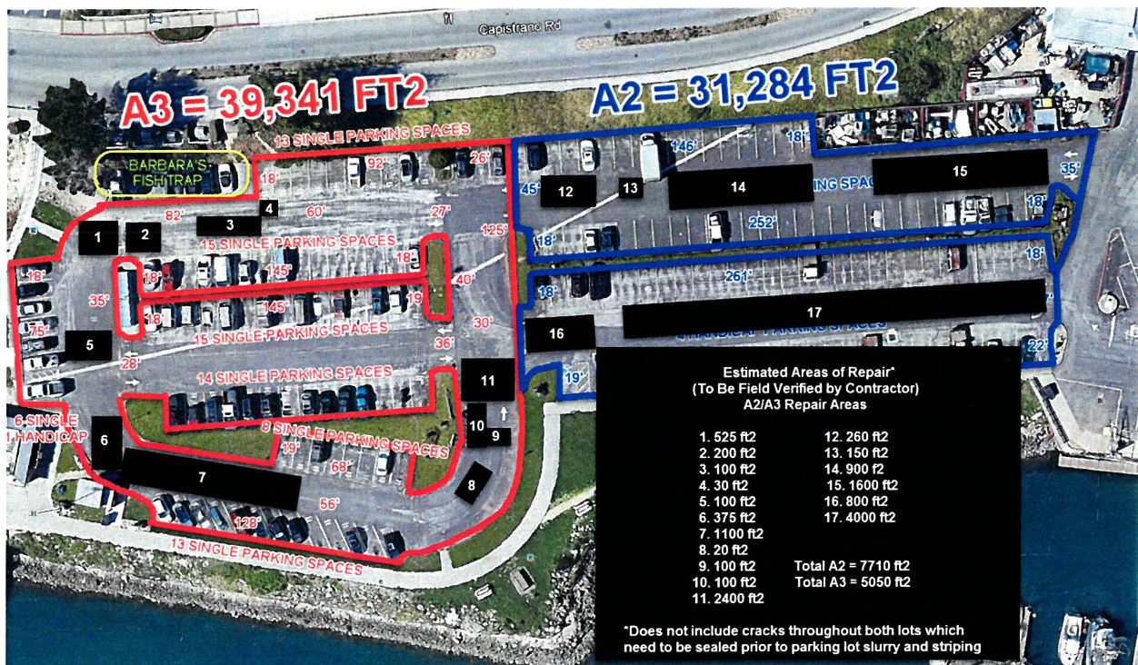
Figure 9 - Large Defective Areas to be Repaired
