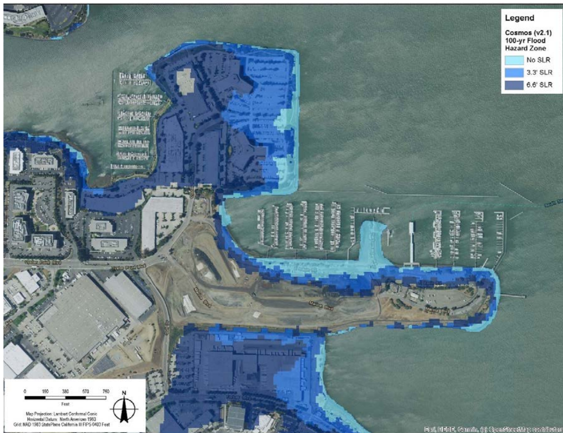
Figure 18. Oyster Point Marina, Flood Hazards for 100-year Event + SLR (Source: USGS)
